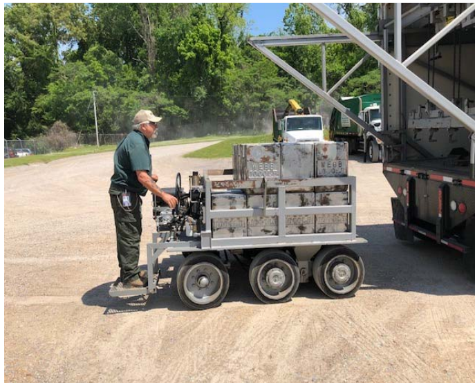
Test cart with test weights are transported back to test truck to reload
