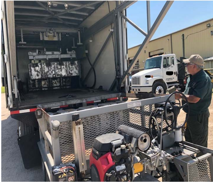
Test weights being loaded into test truck
