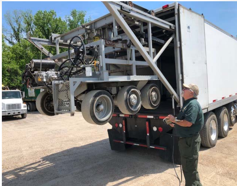
Test cart being loaded into test truck
