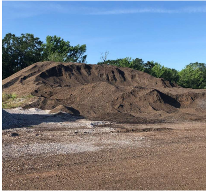
Asphalt milling is reused for other operations
